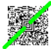
The aiming beam is smaller when the scanner is closer to the code and larger when it is farther from the code. Hold the scanner close to smaller bar codes, and farther away from large bar codes to get a proper read.
